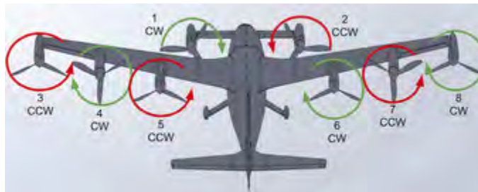
Heaviside Motor/Propeller Names and Rotation Direction
